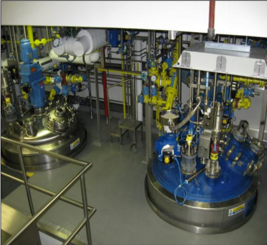
SBV for contained Intermediate Bulk Container (IBC) charging
