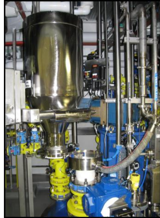
SBV for contained Intermediate Bulk Container (IBC) charging
